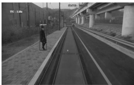
Fig. 10. TTC, Predicted Collision Point &amp; Warning Message
