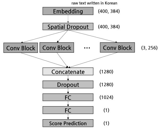
Fig. 2. Overview of Our CNN Architecture for Movie Rating Prediction
