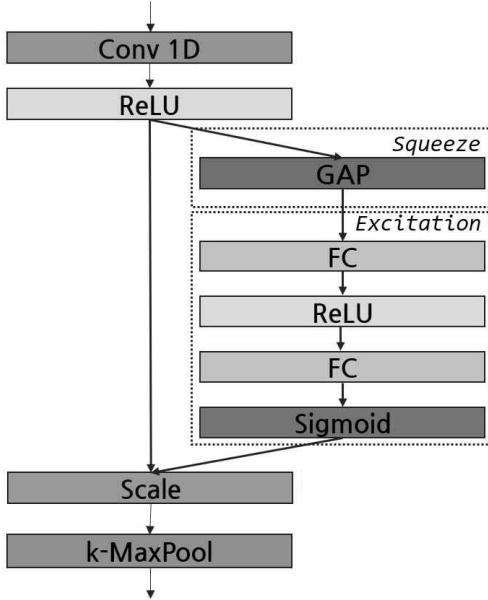
Fig. 3. Convolution Block in Our Network. We Improve the Basic Convolution Block with an SE Block (Dotted Box)
