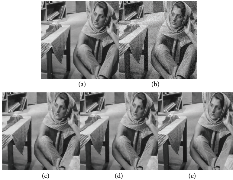
Fig. 4. Image de-noising performance comparison of Barbara image and \sigma = 15 : (a) original image, (b) noisy image, (c) guider filtering, (d) EPLL, and (e) proposed method.
