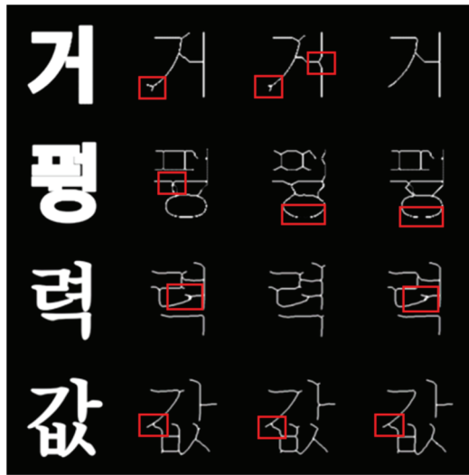
Fig. 1. Problems of existing skeletonization approaches. By column order: ground truth font, skeletons generated by [11], [12], and [13] methods, respectively.
