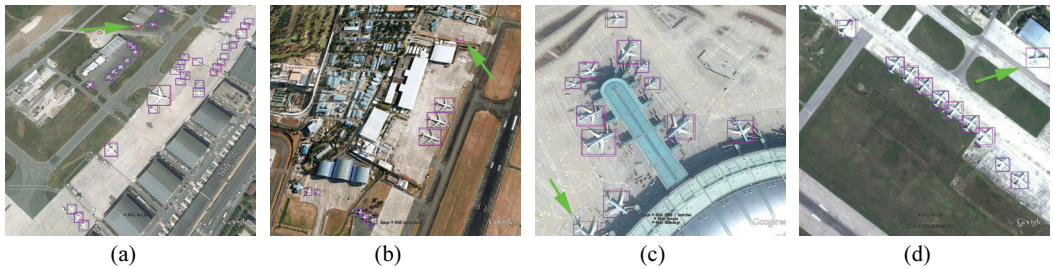
Fig. 8. Experimental results of Inc-v1-Yolov3 on test set: (a, b) smaller aircraft detected, (c) half-price aircraft detected, and (d) aircraft detected in high light.
