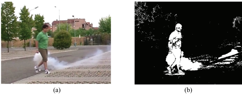
Fig. 1. Moving object detection: (a) screenshot from the video and (b) the moving object.
