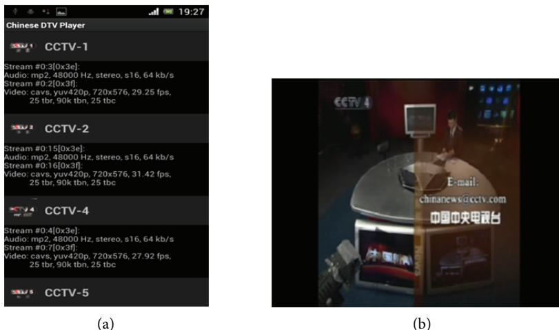
Fig. 9. (a) User interface of parsed program information. (b) DTV rendering example.
