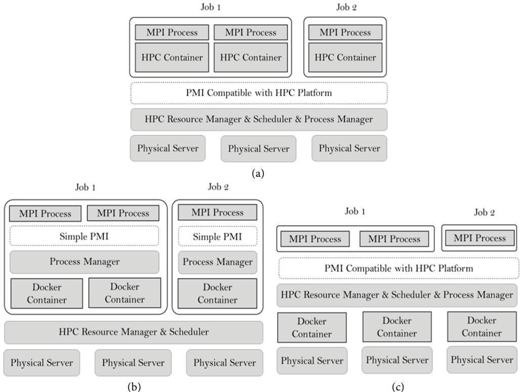
**Fig. 1.** HPC platform structure. (a) HPC container integration with existing HPC platform. (b) Docker case 1: container as MPI process of each job. (c) Docker case 2: container as HPC worker node.
