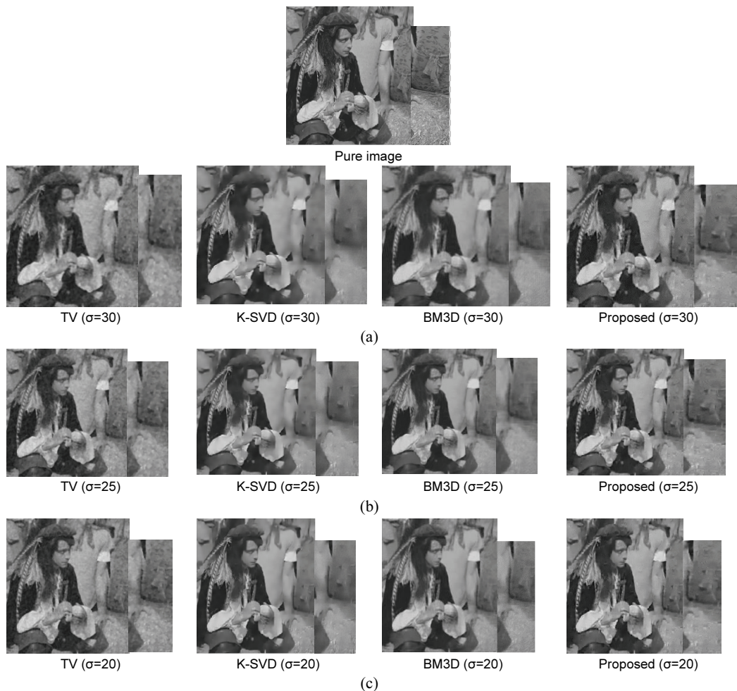
Fig. 4. Denoising image schematic diagram based on different image denoising methods: (a) \sigma=30 , (b) \sigma=25 , and (c) \sigma=20 .
