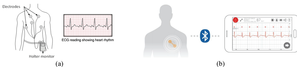
Fig. 1. ECG signal-acquisition devices: (a) a Holter monitor and (b) a Bluetooth-based device.
