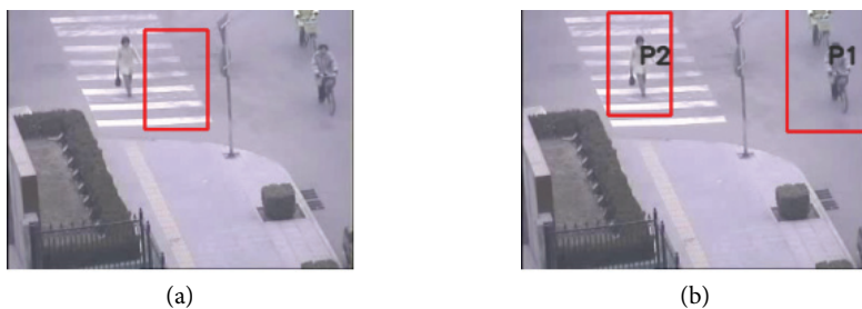
Fig. 14. Correction of tracking error 3: (a) incorrect-mapping error by SURF tracking and (b) correction by the proposed tracking.
