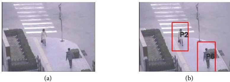
Fig. 12. Correction of tracking error 1: (a) no-mapping error by SURF tracking and (b) correction by the proposed tracking.
