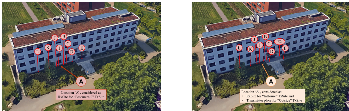
(a) Receiver locations when the transmitter is in sanitation room of the basement (TxSite: 'basement-0'). (b) Receiver locations when the transmitter is inside the building (TxSite: 'InHouse'), or outside the building (TxSite: 'Outside').
