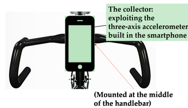
Fig. 18. The collector and the controller : The collector mounted at the middle of the handlebar, head up.
