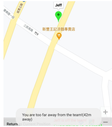
Fig. 10. The mobile app function – off-the-team warning: The off-the-team member (Jeff)'s UI (cropped) with “You are too far away from the team! (42 m away)” indicated at the bottom.
