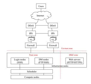
Fig. 7. Service environment of network security construction.
