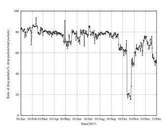
Fig. 5. Ratio of dropped packets by non-matching of firewall rules out of total dropped packets.
