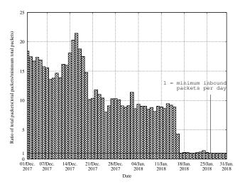
Fig. 9. Traffic volume to be handled by the firewall.
