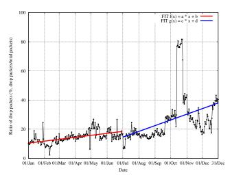
Fig. 3. Ratio of dropped packets out of total dropped packets by the drop rule of the firewall.
