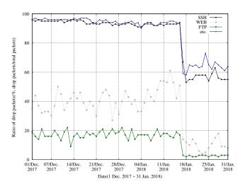
Fig. 11. Ratio of the dropped packets for all services with pre-filtering ACL.
