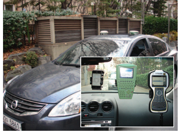
Fig. 3. Positioning system implemented with smartphone and DGPS receivers inside road test vehicle and DGPS antennas outside road test vehicle.
