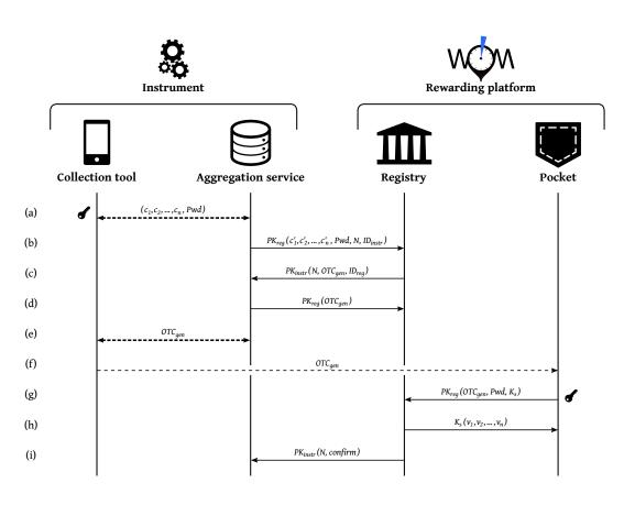
Fig. 2. Diagram of the communication protocol for generating vouchers.
